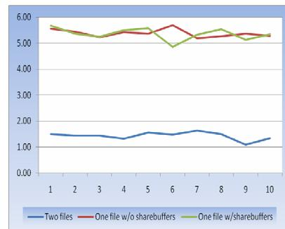
File structures 2 and 3 decrease wall time when the file is not fully defined and only functions are used to update the output data, and increase User and System CPU times at the same time.
