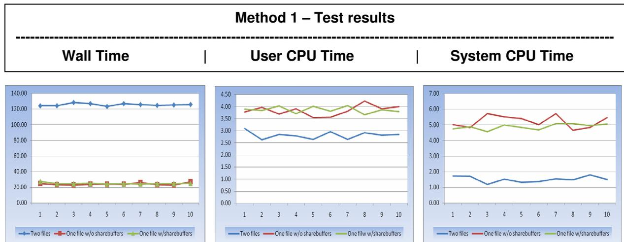
File structures 2 and 3 decrease wall time when the file is fully defined, and increase User and System CPU times at the same time.
