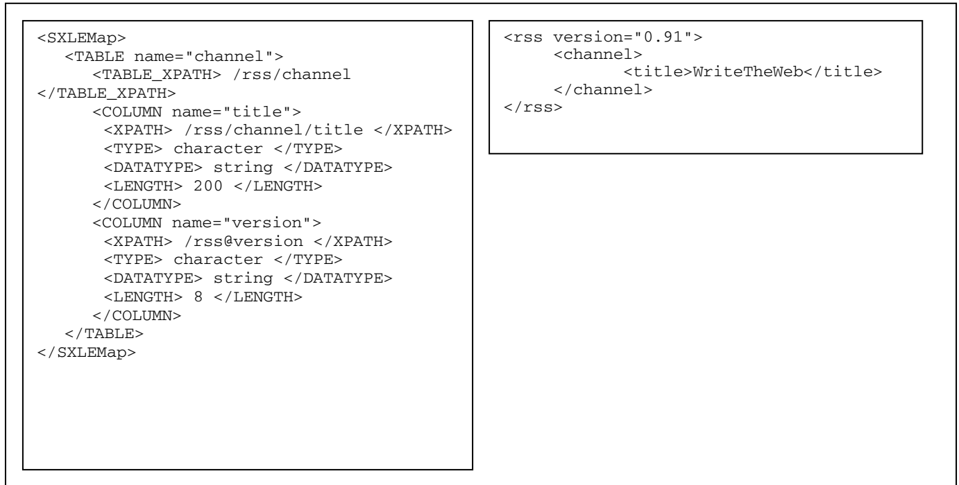
Figure 1. XMLMAP with a Sample of XML
